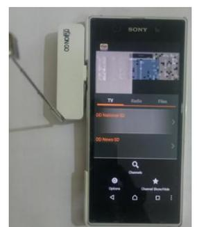
**Android Users:** TV-On-GO Micro USB Dongle (to be used with OTG Enabled Android Smartphone) with mini antenna
